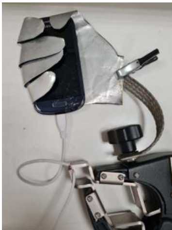
Fig. 6 Measuring the frequency response of the coupling between the victim's hand and the smartphone.
