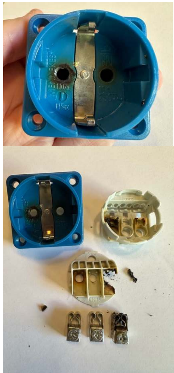
Fig. 2 An overheated Schuko (Type F) socket outlet assembled and disassembled.
