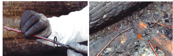
Fig. 1 The floor heating cable was mounted with clamps which depressed the cable (Image: Lapland Police)
