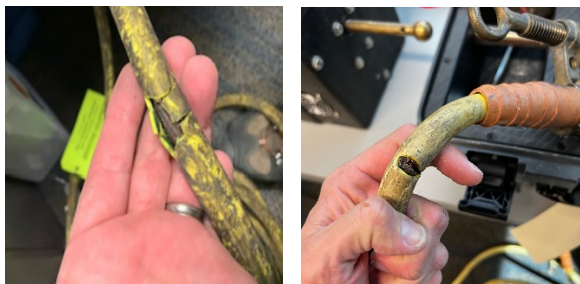
Figure 7 – Example of failed TPGs during visual inspection – defective jacket (left), cut strands (right)
